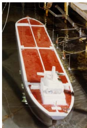
1978 – Mooring tests for Pointe Limboh (Cameroon) with gas and oil tankers at Sogreah's Laboratory.
