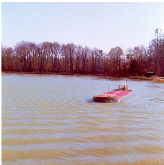
1974 – The Antifer arrives at Port Revel and is subjected to waves generated on the lake (still a unique feature in the world in 2005).
