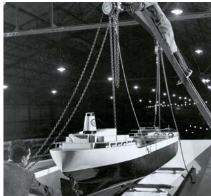
1958 – The Pembrokeshire, then prosaically named PR 1116, a 70 000 t tanker at scale 1/40, later changed into an 18 000 t tanker at scale 1/25.
