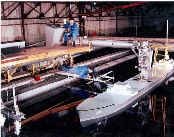
1965 – Again in the Kiel Canal study, the Pembroke is now coupled to a dynamometer to measure forces on the ship.
