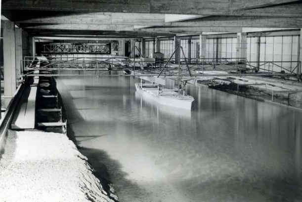
1953 – Probably Sogreah's first ship (at Laboratoire Dauphinois d'Hydraulique): the Sovac Comet, a 30 000 t tanker.
